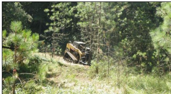
Implementation: Skid steers used shears to cut each tree at ground level. This facilitates later management via mowing.
