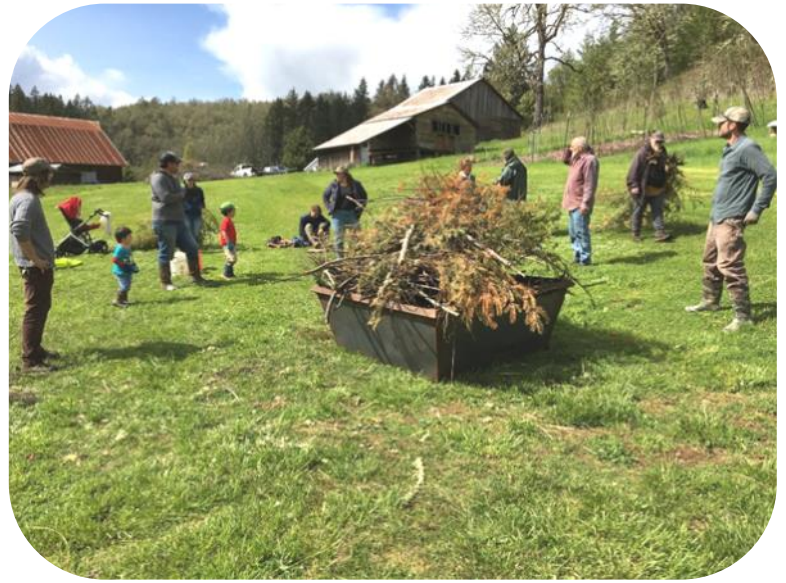
(Above) A group of consultants, landowners, and partners load a steel kiln, "The Oregon Kiln," with Douglas fir and Scotch broom slash to turn it into biochar.
