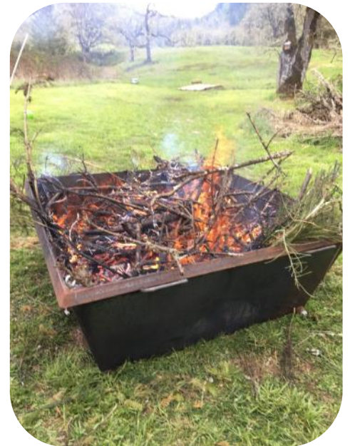
(Below) The small diameter wood quickly transforms into biochar and the fire needs quenching with water to stop the wood from becoming ash.
