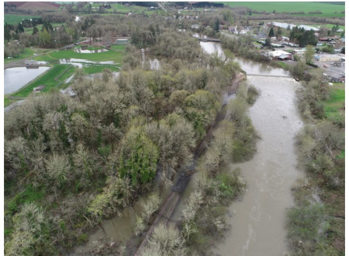
This photo from April 2019 during high flows (~4800 cfs) shows how the drop structure (“dam”) at Monroe slows water briefly but does not store water. It’s called a run-of-river or low-head dam. These dams create drowning hydraulics such that many states are actively removing them, and the one at Monroe is a fish passage barrier under almost all conditions to some of our most iconic and valuable fish. This great shot by Clinton Begley’s drone also highlights the side channels and slough habitat. Thanks to the many landowners and community members continuing to work to reconnect and restore habitat throughout the watershed.
